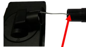
Pass the cable into the first tube
