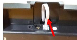
Insert cable into the connector
